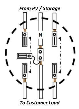
120/208V & 120/240V Single-phase, 3-wire 5-terminal meter socket 400 amp or less
